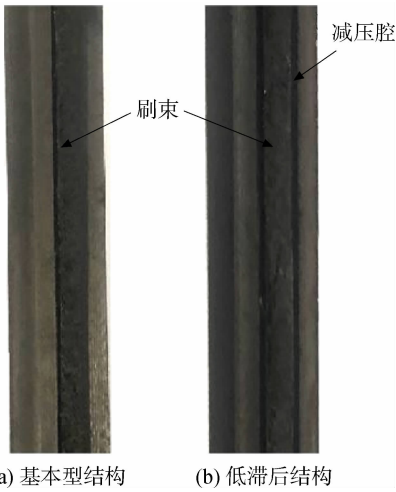
图 4 基本型和低滞后刷式密封试验件内环面局部对比图 Fig. 4 Comparison of inner surface between conventional and low hysteresis brush seals
